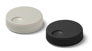
The knob in  $\emptyset$ 33 mm is fixed with screws. The knob is suitable for  $\emptyset$ 6 mm shafts and available in the colours grey and black. The recessed grip and the ribbed edge give the knob a secure haptic appearance.
