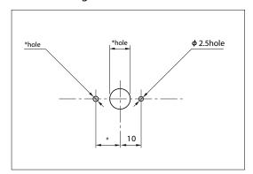
Note: The diameter of \*hole is depending on the diameter of potentiometer to be mounted
