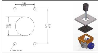
The joystick is mounted from below. The frame has M2.5 tapped holes.
