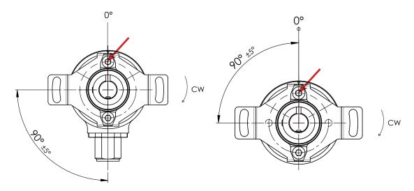
(\*) The drawings above shows the zero degree (0°) reference If the shaft slot is in a line with the groove in the encoder housing (groove is marked with a red arrow) then the output signal is 0% full-scale.
