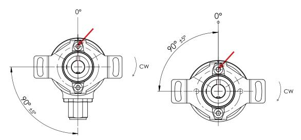
(\*) The drawings above shows the zero degree (0°) position If the shaft slot is in a line with the groove in the encoder housing (groove is marked with a red arrow) then the output signal is 0% full-scale.
