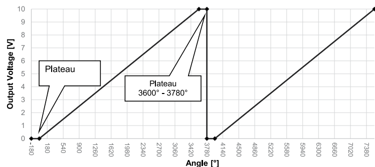
The drawing shows the signal amplitude function for 0 to 10 V signal output
